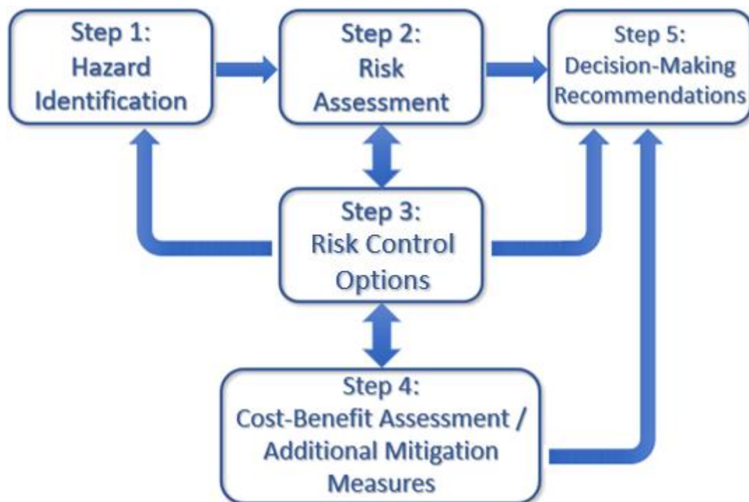
Figure 3-1 Flow Chart of the FSA Methodology (IMO, 2018)
